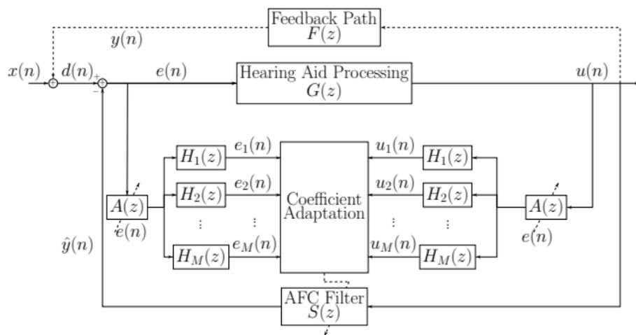
Figure: Block diagram of the proposed AFC framework.
